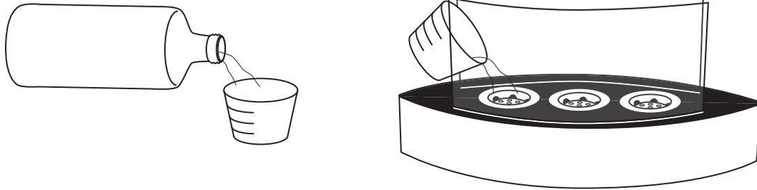
Using the measuring cup provided (Part D), carefully measure 150 ml of **liquid ethanol fuel for fireplaces** and pour it into each burner. **If any fuel does spill, you should always wipe it up prior to lighting your fireplace.**
