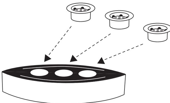
Put fireplace body (Part A) on a steady surface and insert the 3 burner cups (Part C) into the holes on the fireplace body.
