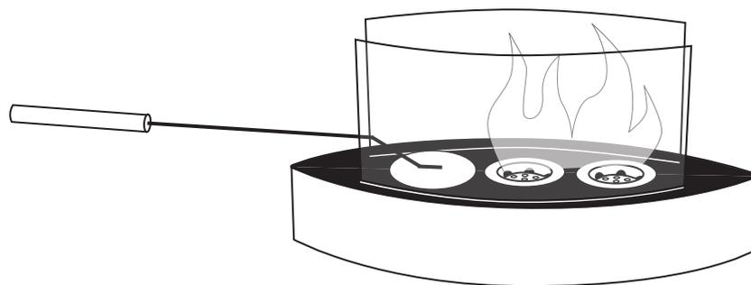
When finished using the fireplace, the handle provided (Part E) should be placed over each burner cup to cut off the oxygen supply to the fuel. This will snuff out the flame.
